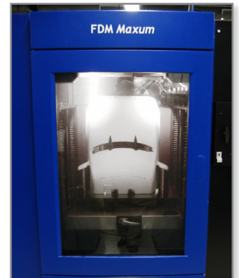
Figure 7: 1/4 scale model of a Jeep Cherokee built on FDM Maxum
