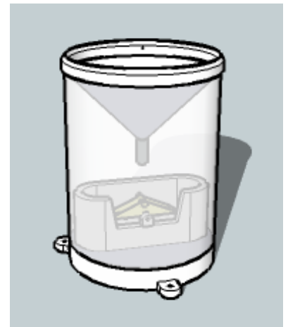
A standard tipping bucket rain gauge used to measure rainfall.
