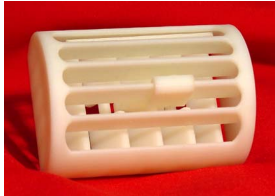
The air vent, constructed as a one-piece assembly, illustrates rapid manufacturing's ability to consolidate parts.
