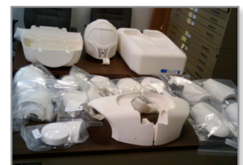
Components for R2 mockup were made by RedEye On Demand digital manufacturing service.
